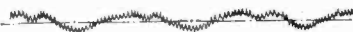
Fig. 1. Hum and noise output from microphone pre-amplifier, using SP41 valve with 100k\Omega resistor between grid and earth.
